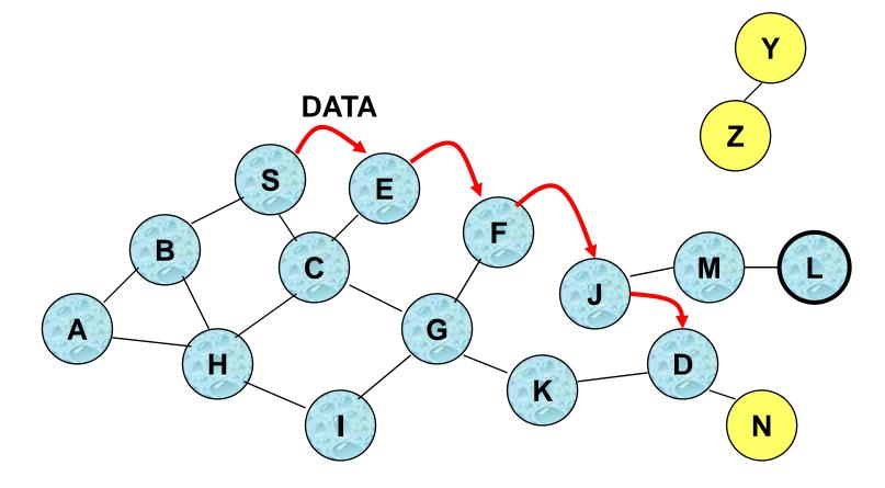
Routing table entries used to forward data packet.
