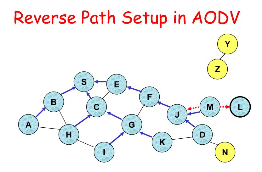
Node D does not forward RREQ, because node D is the intended target of the RREQ
